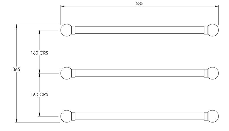
DO NOT SCALE DRAWING ALL DIMENSIONS ARE IN MILLIMETERS AND MAY VARY ± 5mm AS THEY ARE HANDMADE, HAND SOLDERED AND POLISHED WE THEREFORE RECOMMEND THAT ANY INSTALLATION WORK BE CARRIED OUT UPON RECEIPT OF RAIL.
